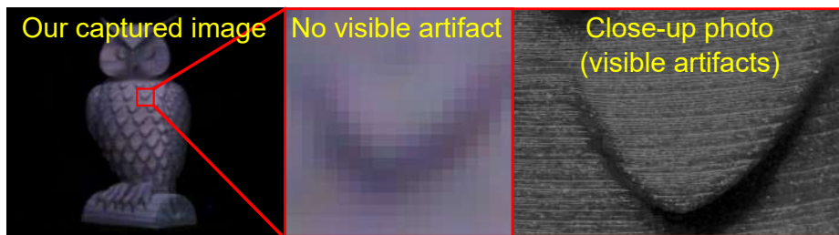
Figure S4. 3D-printing error. 3D-printing artifact is too small to be observed in our captured image. It can be observed in a close-up photo.
